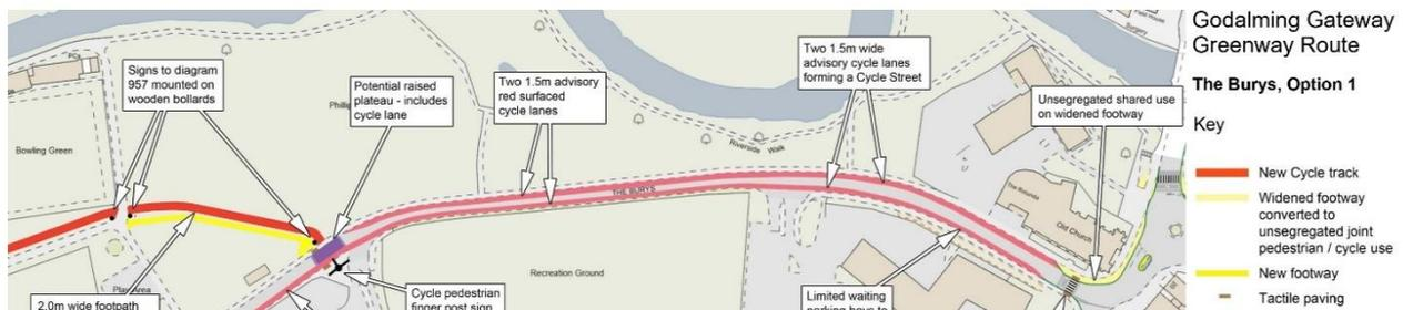
Figure 4: The Burys on-carriageway option proposes a 'cycle street' approach. This would see the centre line removed and replaced by advisory cycle lanes each side of a central motor vehicle lane. It avoids the need for a shared-use path at the eastern end of the route where pedestrian footfall is highest.
